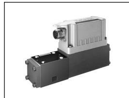
4WRPEH 6 is a high performance, direct operated, servo-solenoid valve. It is suitable for closed loop applications like position, velocity, and pressure control. It is even more robust than the previous desgin. Series-3X is not designed for pilot operated applications, 3WRCBH, or 4WRLE.
