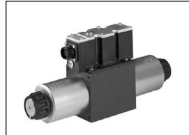
The WRA(E) direct operated proportional valve without integral feedback is available with or without on-board electronics (OBE). Individual valve amplifiers are available for the non-OBE version. Postive overlap spools reduce leakage at center and OBE models can be configured to either a voltage or current command.
