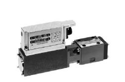
DREBE6X is a pilot operated pressure reducing/relieving valve for high performance applications. Pressure in port A is controlled by a proportional solenoid using position feedback with on-board electronics (OBE).
