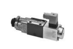
DBETFX proportional pressure relief valves are direct operated valves with position feedback for limiting system pressure. The position of the valve cone is measured by the Lvdt AC/AC position transducer, and the position of the cone-solenoid position is controlled by external trigger electronics, resulting in a linear curve.
