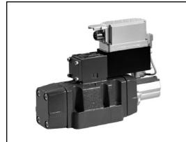
Pilot operated proportional directional valve type 4WRLE offers integral position greater feedback on both pilot and mainstage for dynamic response plus greater accuracy. On-board electronics (OBE) and 7-pin connectors permit power and command all to be accomplished on the valve. Overlapped main spools and high-performance pilot permit application into various circuits including those requiring closed-loop control of pressure, force, or velocity.
