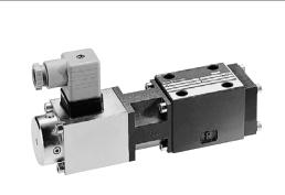
Type DBE6X proportional pressure relief valves are pilot operated pressure relief valves. The valves are actuated by means of a proportional solenoid. With these valves, the system pressure that needs to be limited can be infinitely adjusted in relation to the solenoid current.
