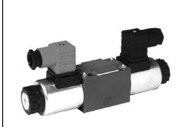
4WRAB6 type direct operated proportional valves are available with or without on-board electronics (OBE). Suitable for open loop applications, the WRAB6 does not have integral feedback; however, provides proportional flow output dependant on a commanded value. The WRAB6 may also be used with a DC switching signal, if the application requires throttled shifting without full proportional control.
