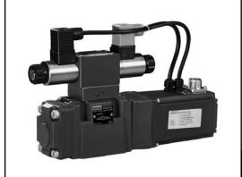
The 4WRKE is a pilot operated proportional directional valve with position feedback on the main stage. The onboard electronics (OBE) has a standard 7-pin connector for command, spool feedback, and 24V power. Overlapped spools have a spring centered fail-safe position. 4WRKE is normally used for open loop applications where higher repeatability is more important, also for lift, transfer, or clamping applications.
