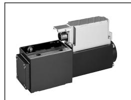
The 5WRPE 5/3 high-response directional control valve is a directly operated component. The valve is actuated by control solenoids with integral position feedback and on-board electronics. Electronics are factory-calibrated.
