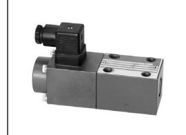
DBETX proportional pressure relief valves limit pressure for piloting applications. Pressure is limited by changing current to the proportional solenoid from an external amplifier.
